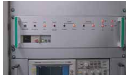
Figure 5. The LDS-Dactron Laser controller is integrated into a 19" instrumentation module, together with the main indicators to monitor the operation of the shaker.
